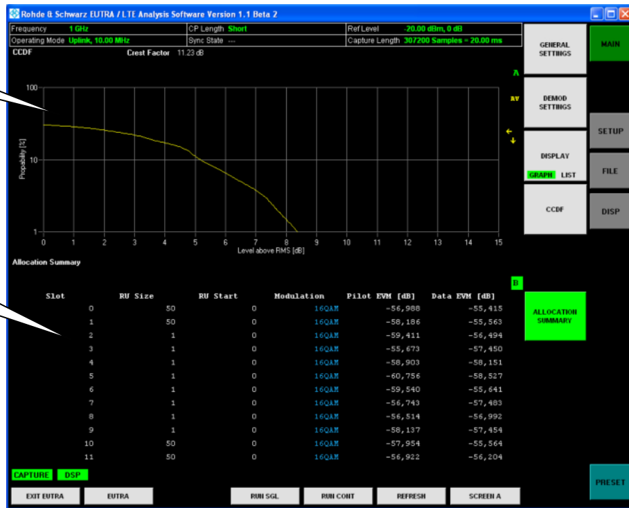
Figure 5-17 Analyzing EUTRA/LTE UL signals – CCDF and Allocation Summary
